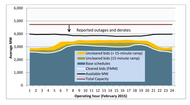
Figure 4.3 Average schedules, bids and dispatches by operating hour – February 2015 PacifiCorp East - 15-minute market (gas and coal units)
