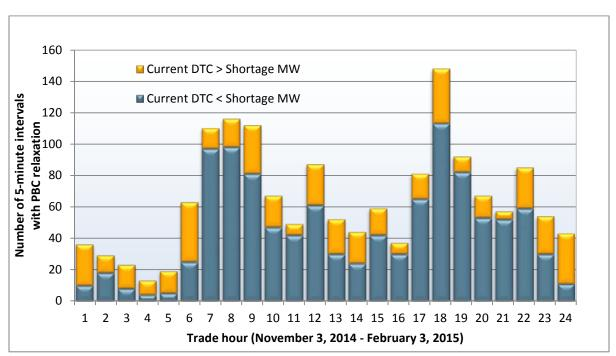
Figure 6.1 Potential power balance relaxations in 5-minute market mitigated by new DTC limits PacifiCorp West (November 3, 2014 through February 3, 2015)
