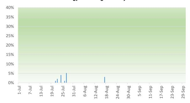
Figure 29: Frequency of flexible ramping sufficiency test failures in the PAC West balancing authority area
